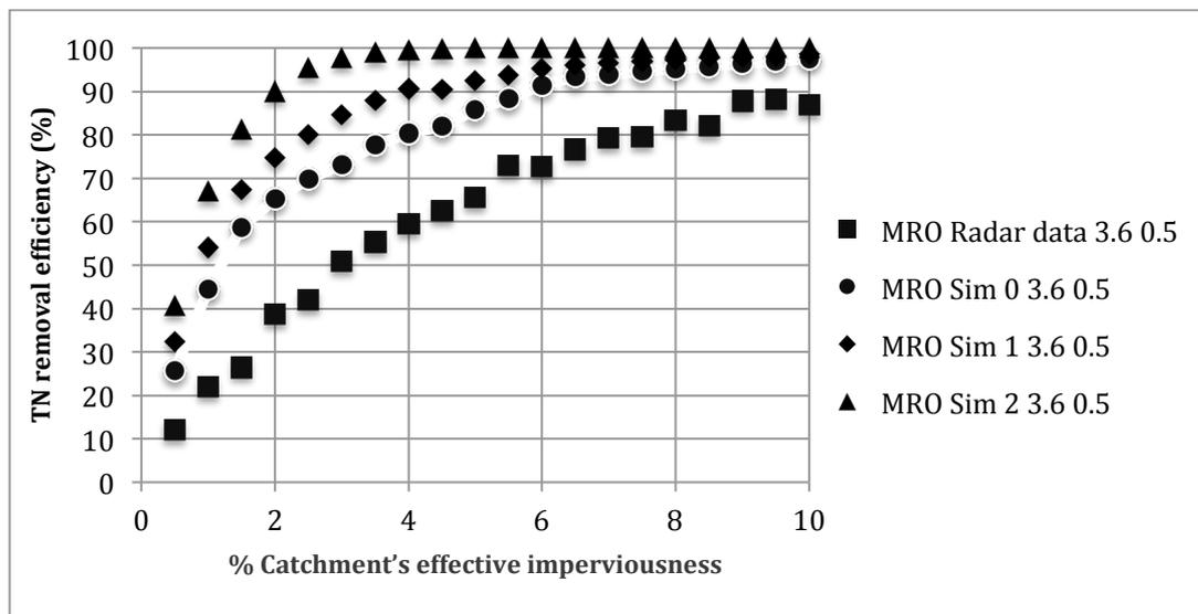
**Figure 1.** TN removal efficiency estimates according to radar rainfall and three modelled rainfall timeseries for wetlands in the Melbourne Regional Office location with an exfiltration rate of 3.6 mm/h and an extended detention depth of 0.5 m.
